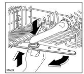
Slide out the upper basket. Push downwards on the water feed pipe, simultaneously push the spray arm upwards and turn it in a clockwise direction.
